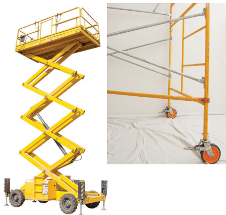
Scissor lift (left) and mobile scaffold.
