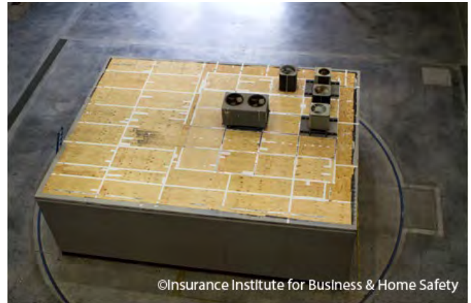
AC units in the above picture were used during recent tests, which included a specific focus on wind load specifications and future prescriptive guidelines for anchorage.
