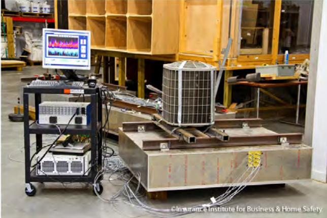
The picture above shows some of the tools that allow IBHS to measure various loads on AC units during tests.
