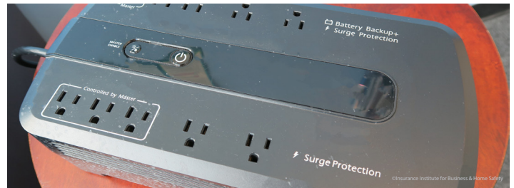
A surge suppressor, or surge protector, like the one pictured above can protect equipment from electrical surge damage.
