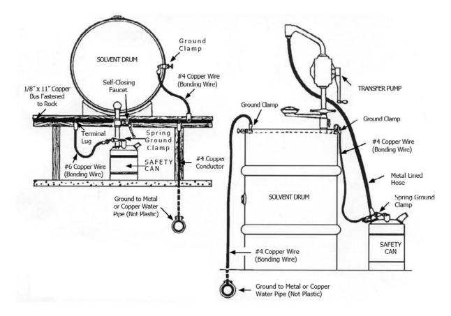
The NFPA illustrations above show grounding of solvent drums and methods of bonding drums to small containers being filled. If a good electrical connection is known to exist from the drum to the can through a metal lining and nozzle of the hose, the bonding cable between the drum and the container is not required.
