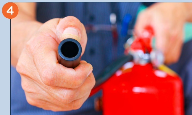
4 For Maximum Effectiveness: Aim the Nozzle at the Base of the Fire
