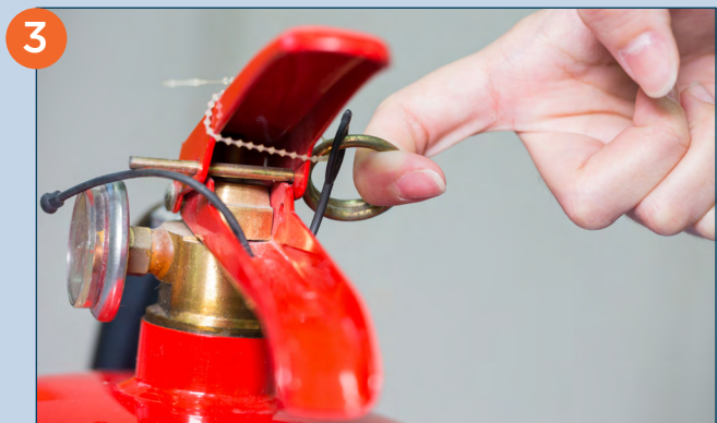
3 In the Event of a Fire: Begin By Pulling the Pin Near the Top of the Tank
