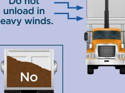
Tipping occurs when the center of gravity moves as the bed is raised.
