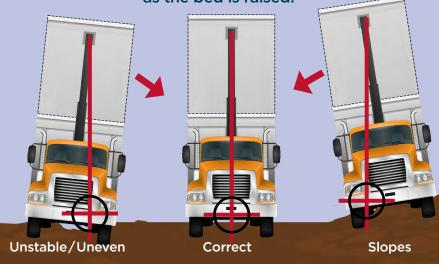
Unload on flat stable ground. Slopes or unstable ground can create major shifts in the center of gravity and rollovers.
