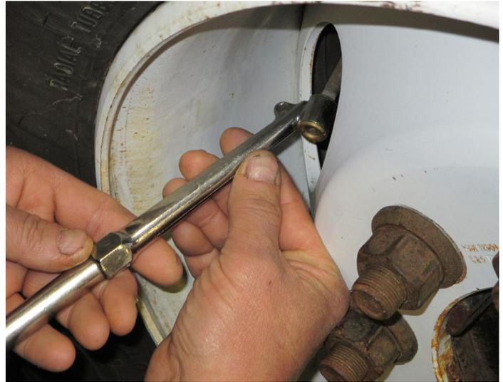
**“Thumping” tires does not accurately measure tire pressure. Tire pressures should be measured using a commercial-grade tire pressure gauge.**
