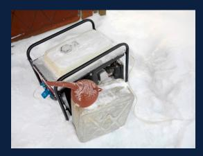
Snow accumulation on a generator, as shown above, can significantly impact performance during a snow storm.
