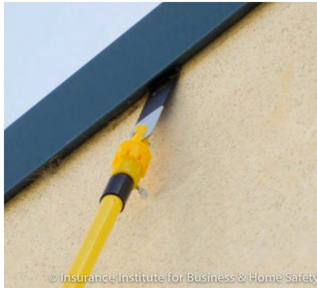
A flashing inspection tool developed by IBHS allows an inspector to physically check the flashing from the ground.
