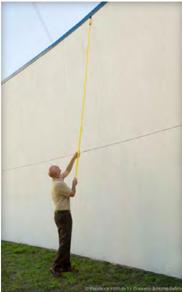
A flashing inspection tool developed by IBHS allows an inspector to physically check the flashing from the ground.
