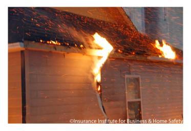
Above is debris that ignited in a vinyl gutter during a wildfire ember storm demonstration at the IBHS Research Center. If in a wildfire-prone region, use metal gutters and downspouts and regularly remove debris from gutters.
