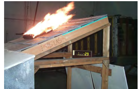
Test to determine the fire rating for a roof covering. A Class A burning brand is on this roof covering. Photo taken during experiments conducted at the University of California Fire Research Laboratory. Source: Stephen L. Quarles
